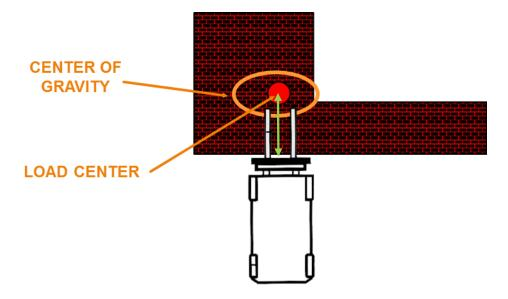
The load center is the distance from the carriage, or vertical face of the forks, to the center of gravity of the load. In the examples below the load centers are:
