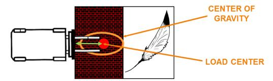
Similarly, the center of gravity for odd shaped loads of similar materials will be near the side with the most mass.
