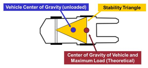
Keeping the downward force of the load (center of gravity) within the stability triangle keeps the forklift stable and keeps the load for crashing to the ground. Allowing the load to move outside the stability triangle makes both the forklift and load less stable and subject to tipping, rolling, or dropping.
