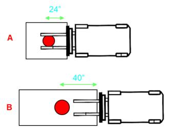
So understanding the center of gravity and load center help the operator to determine how to pick up a load and maintain stability (pick up the load on the side closest to the center of gravity). In example B above, the load should be picked up from the side, not the end as shown.
