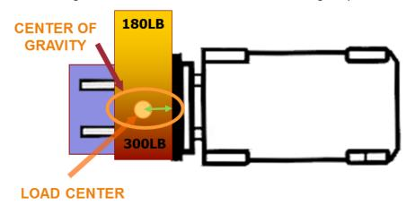
If a load contains materials with different weights or densities, the center of gravity will be on the side containing the heavy material. For example: If a pallet contains bricks on one side and feathers on the other, the center of gravity will be closer to the side of the pallet containing the bricks.
