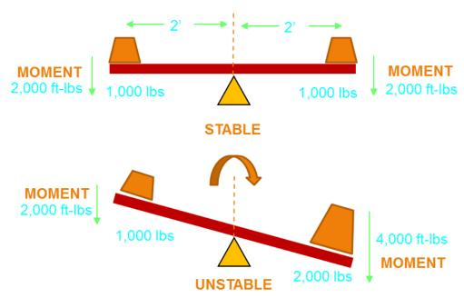
From that bit of knowledge, let's define a couple of more terms that will help us determine the stability of a forklift. Earlier we mentioned center of gravity and load center. The center of gravity is the average location of the weight of an object. The load center is the distance from the carriage, or vertical face of the forks, to the center of gravity of the load.
